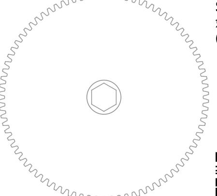
\$2,500 First Gear – 84 tooth, ½ inch thick, 4.3" in diameter (all gears printed at actual size)
